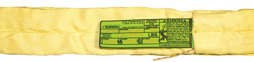
Use only if trained. Do not exceed rated capacity. Protect sling from being cut by load edges, corners, protrusions and abrasive surfaces. Avoid exposure to acid, alkali and temperature over 300°F. DEATH or INJURY can occur from improper use or maintenance.
