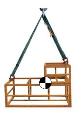
The Twin-Path<sup>®</sup> Adjustable Bridle should be used where the double leg horizontal angle is greater than 45°. Always connect above the center of gravity. If connections are made below the center of gravity, then the load may turn while lifted.
