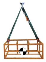
If one of the lifting points is closer to the center of gravity, then attach the double leg to this lifting point. It will have the highest weight concentration. If the Twin-Path<sup>®</sup> Adjustable Bridle is attached so that the single leg is nearest the center of gravity, the lift cannot be made.
