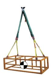
**WARNING** Slings can fail if damaged, misused or overloaded. Inspect before use. Damaged slings shall not be used. Use only if trained. Do not exceed rated capacity. Protect sling from being cut by load edges, corners, protrusions and abrasive surfaces. Avoid exposure to acid, alkali and temperature over 180°F. DEATH or INJURY can occur from improper use or maintenance.
