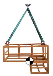
If the lifting points are an equal distance on either side of the center of gravity but one is higher, then the double leg should be attached to the higher lifting point.
