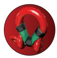
The pin area of a shackle can damage synthetic slings. Placing synthetic slings on the pin should be avoided. Shackles may have a sharp edge where the pin goes through the shackle ear. If the sling is rigged on this area, it could become severely damaged. If you must rig on the pin, protect your sling with a **Shackle Pin Pad**.
