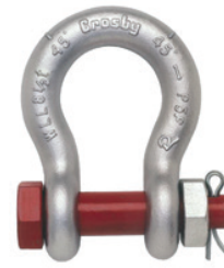
G-2130/S-2130 Bolt Type Anchor shackles with thin head bolt - nut with cotter pin. Meets the performance requirements of Federal Specification RR-C271G, Type IVA, Grade A, Class 3, except for those provisions required of the contractor.
