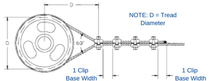
If a pulley (sheave) is used, in place of a thimble, add one additional clip. Clip spacing should be as shown.
